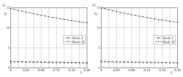
Fig. 6. The imaginary part of the roots of characteristic equation (2.34),  $\gamma = 0.5$ ,  $\alpha = 1$ ,  $\beta = 0.005$ : (a)  $\tilde{\mu}_{\gamma} = 0.008$ , (b)  $\tilde{\mu}_{\gamma} = 0.016$
