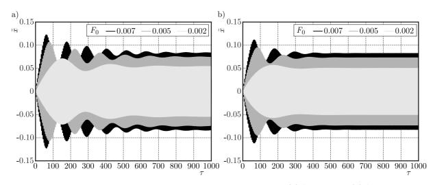
Fig. 10. Nonlinear beam response, harmonic excitation,  $\gamma = 0.5$ : (a)  $\tilde{\mu}_{\gamma} = 0.008$ , (b)  $\tilde{\mu}_{\gamma} = 0.016$
