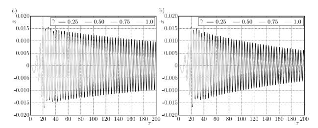
Fig. 9. Nonlinear beam response, transient excitation,  $\mathcal{E} = 0.1$ ; (a)  $\tilde{\mu}_{\gamma} = 0.008$ , (b)  $\tilde{\mu}_{\gamma} = 0.016$
