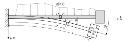
Fig. 1. Schematic of the analyzed beam
